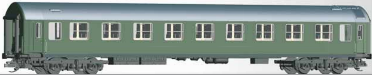
Reisezugwagen 1./2. Klasse, Typ Y, der DR 1st/2nd class passenger coach, type Y, of the DR
