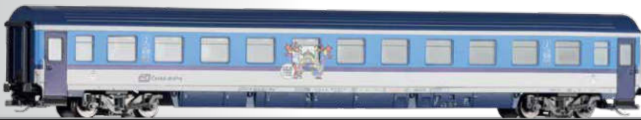
Reisezugwagen 2. Klasse mit Kinderabteil, Bmz 229, der ČD 2nd class passenger coach with children's compartment, Bmz 229, of the ČD
