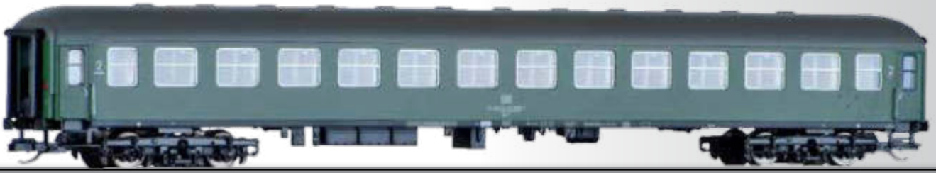
Reisezugwagen 2. Klasse Bm 232 der DB 2nd class passenger coach Bm 232 of the DB
