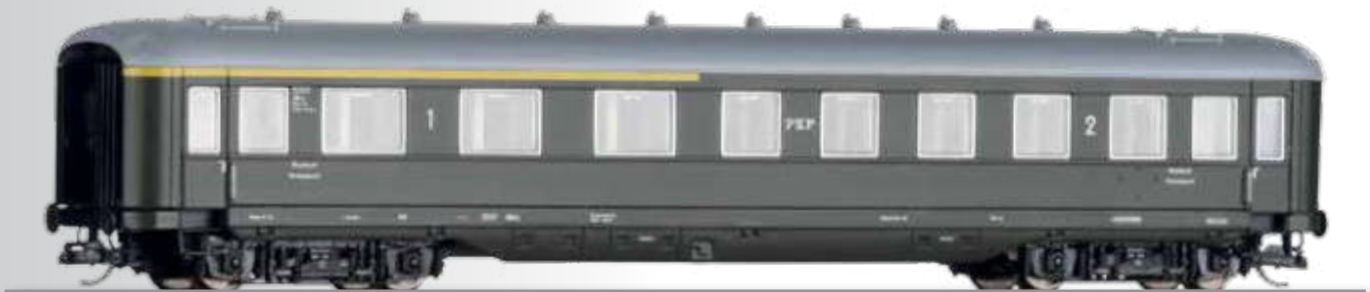
Reisezugwagen 1./2. Klasse ABhxz der PKP 1st/2nd class passenger coach ABhxz of the PKP
