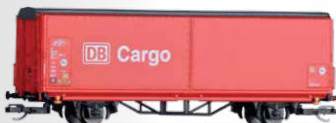
Schiebewandwagen Hbis-tt 293 der DB Cargo Sliding wall box car Hbis-tt 293 of the DB cargo
