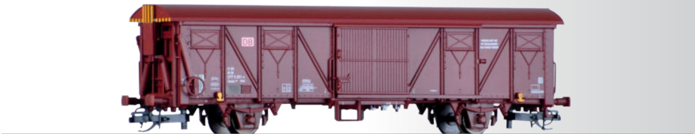
Schwenkdachwagen Tbekks 846 der DB AG Swing roof car Tbekks 846 of the DB AG
