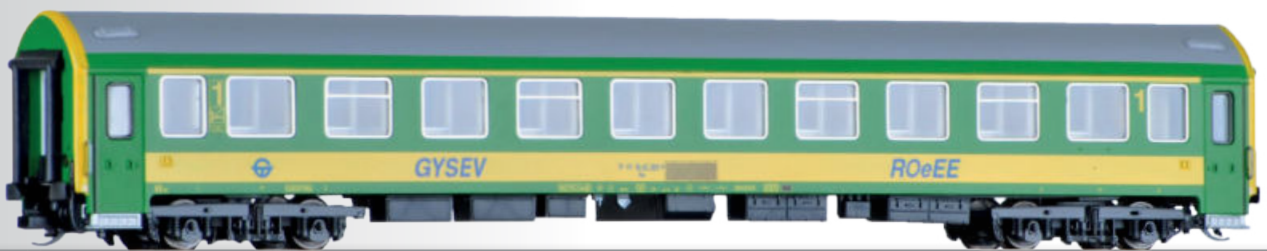
Reisezugwagen 1. Klasse Ap, Typ Y/B 70, der GySEV 1st class passenger coach Ap, type Y/B 70, of the GySEV
