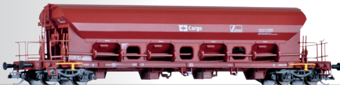
Schwenkdachwagen Tadgnss der ČD Cargo Swing roof car Tadgnss of the ČD Cargo
