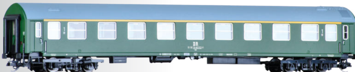
Reisezugwagen 1. Klasse Ame, Typ B, der DR 1st class passenger coach Ame, type B, of the DR
