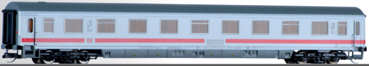
Reisezugwagen 1./2. Klasse Abvmz 111.2 der DB AG 1st/2nd class passenger coach Abvmz 111.2 of the DB AG
