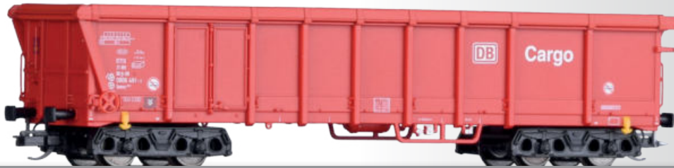
Rolldachwagen Tamns 893 der DB Cargo Sliding roof car Tamns 893 of the DB Cargo
