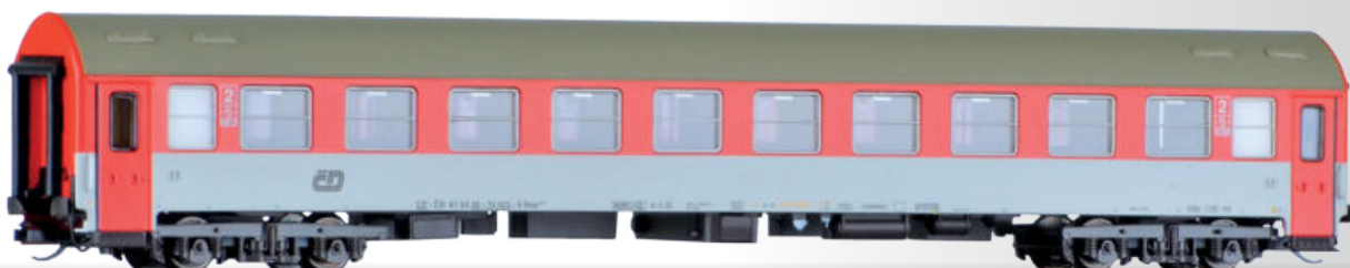
Reisezugwagen 2. Klasse Bee, Typ Y/B 70, der ČD 2nd class passenger coach Bee, type Y/B 70, of the ČD
