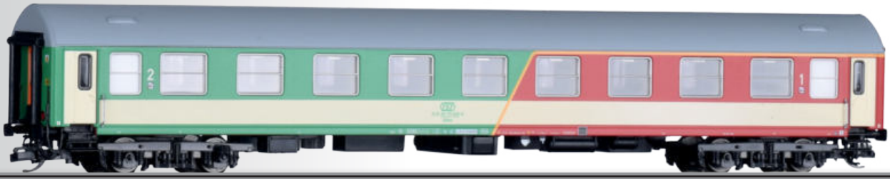
Reisezugwagen 1./2. Klasse ABdnu, Typ Y/B 70, der PKP 1st/2nd class passenger coach ABdnu, type Y/B 70, of the PKP
