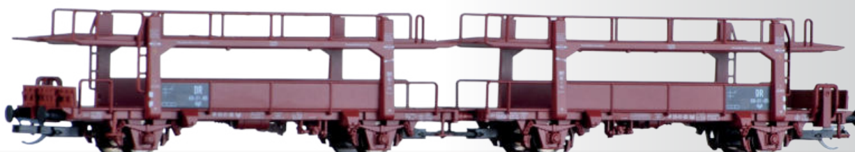
Autotransportwagen Ogll der DR Cars for automobile transport Ogll of the DR
