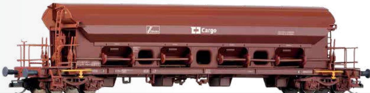
Schwenkdachwagen Tdgnss der CD Cargo Swing roof car Tdgnss of the CD Cargo
