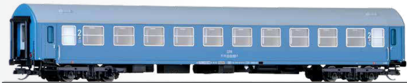
Reisezugwagen 2. Klasse, Typ Y/B 70, der CFR 2nd class passenger coach, type Y/B 70, of the CFR
